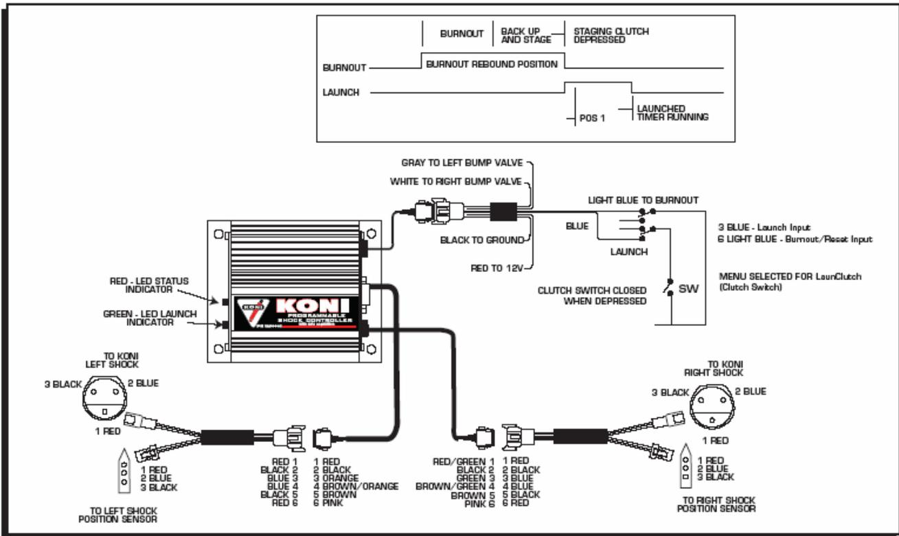
Figure 2: Wiring a Launch/Burnout through the Clutch Switch.
