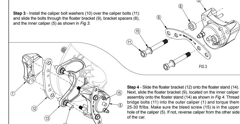
**NOTE**: When the pin in the center of the caliper is almost flush with the caliper housing, its time to change the pads. Do not operate car beyond that point, or fluid loss and brake failure will result. When worn, the inner caliper pad can be resurfaced to become a new outer pad and this service is offered at no charge.
