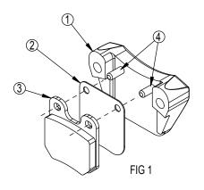
**Step 1** - Install the insulator plate (2) and outer brake pad (3) by sliding them onto the brake pad pins (4) located in the outer caliper (1), as shown in *Fig 1*.
