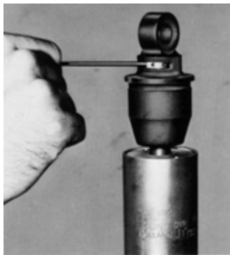
Figure 1: Move pin left or right to increase rebound forces (counter-clockwise)
